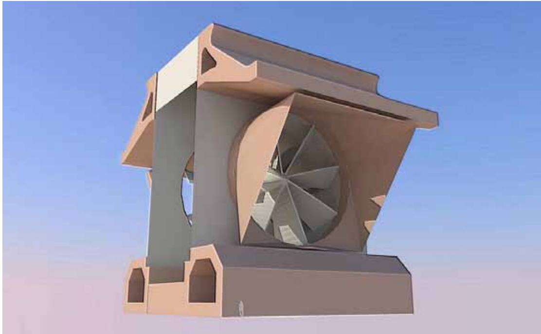
Schematic view of a 20 metre reef turbine (man to same scale)
